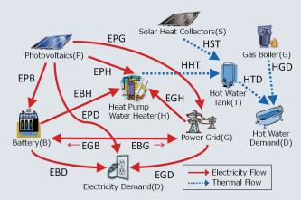
Fig. 2 Targeted appliances and energy flow
