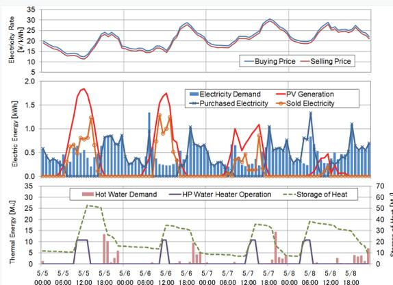
Fig. 3 Optimizing operation of heat pump water heater by using variable power rates
